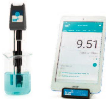
The TRUEscience cap is ideal for measuring up to six different parameters at the same time. It simply clips onto your beaker and can measure pH, Redox, Dissolved oxygen or specific ions simultaneously on an Android Tablet
