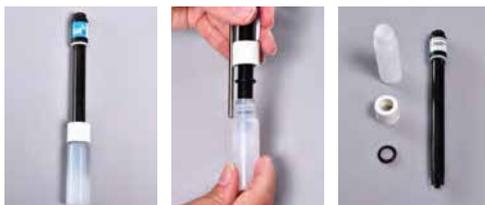
1. Hold the white cap and unscrew the electrode soaker bottle. Move white lid up electrode, pull rubber seal down over electrode tip, then remove lid.
