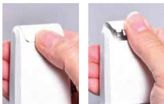
1. Remove the battery cover by placing your thumb on the indented portion on the rear of the battery cover and gently pressing in an upward motion.
