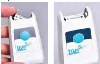
2. Insert the new 1/2AA Li-Thionyl Chloride battery in the slot at the top of the unit. When looking at the front of the unit the positive terminal of the battery should be on the left. See internal guide symbols.
