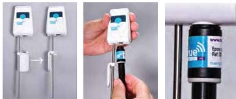
2. Turn the clip attached to the temperature sensor to the left by 90 degrees. Carefully align and screw the pH electrode into the large socket on the base of the unit. Ensure that the electrode is straight and screw gently into the unit. Do not force the electrode as this may damage the thread. Tighten so that the seal is compressed.
