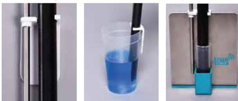
3. Now turn the clip 90 degrees to the right so it clicks over the electrode body. Adjust the height of the clip to suit the size of your container. The clip can be used to attach the unit onto most small beakers and the storage stand. Ensure you have sufficient volume in your beaker to balance the unit.
