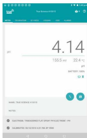
4. Repeat until all buffers have been used. Rinse the electrode between each reading. If icon does not turn green replace your buffers and ensure your rinse step is adequate.
